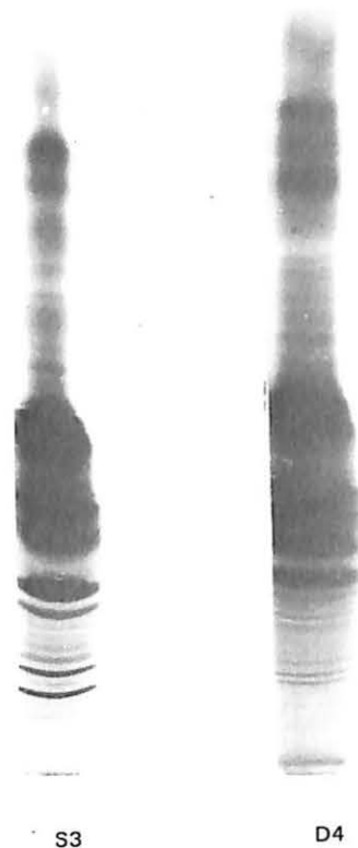
Fig. 6—Composition of semolina (S3) and flour (D4) proteins solubilized with soap (SDS-PAGE electrophoresis).
