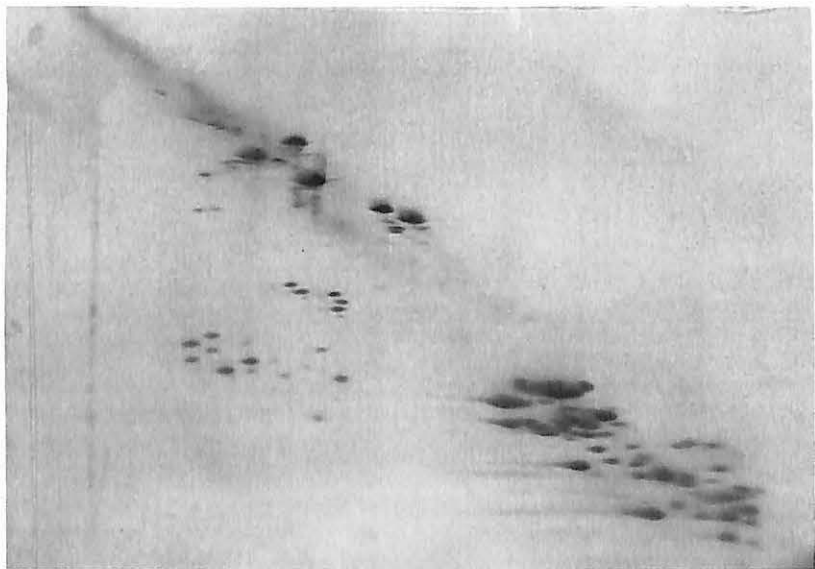
Figure 8 New two-dimensional A-PAGE \times SDS-PAGE electrophoresis for detailed description of LMW subunits in wheat cultivars (from Redaelli, Istituto Sperimentale per la Cerealicoltura, Italy).
